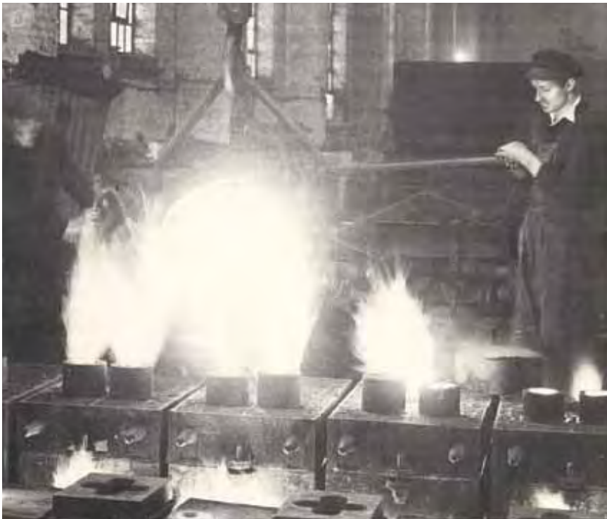
Casting of small items on the floor. We can see that the moulds are filled with molten iron from the ladle that is handled by two men. The gases in the filled moulds are burned off.
