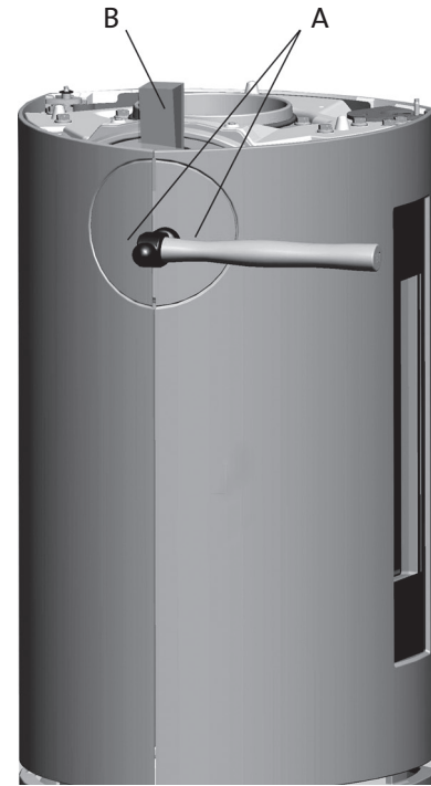
Figure 10. Removing the rear exit outlet knock-outs.
