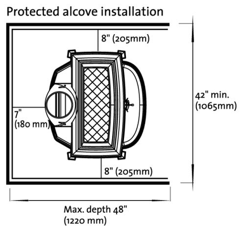
Protection and air space must comply with NFPA 211OR CAN/CSA-B365.
