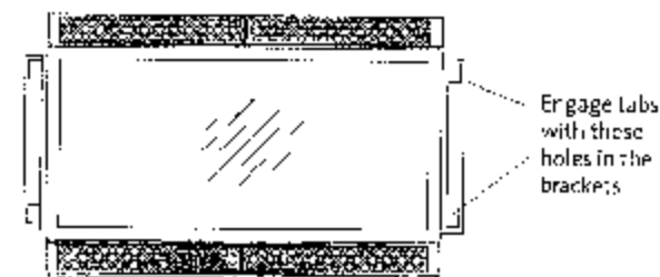
Figure 26. Surround engagement with firebox.
