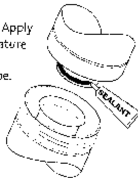
Figure 9. Seal each inner joint before joining pipe.
