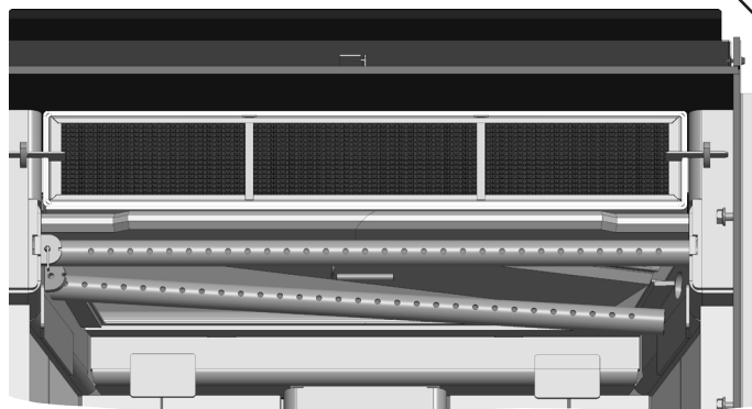
Figure 3.12. Remove the rear air tube by sliding to the right and pulling out.
