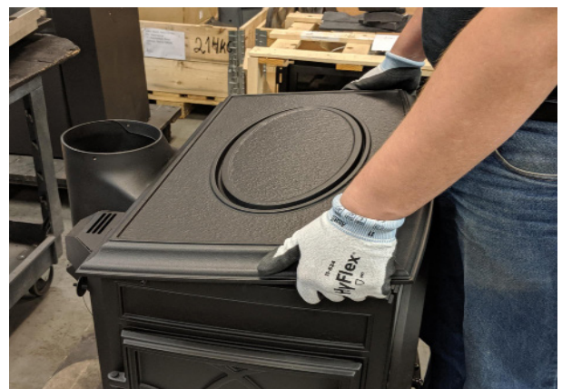
Fig. 21. Remove the top plate from stove.
