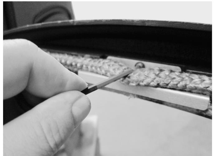
Figure 20. Loosen the glass clips.
