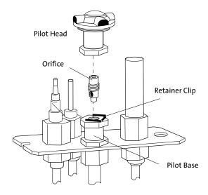
Figure 16. Pilot orifice removal and replacement.
