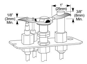
Figure 28. Proper pilot flame appearance.
