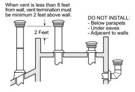
Figure 5. Termination Height Requirements.
