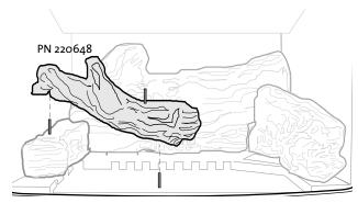
Figure 23. Install Left Middle Log
