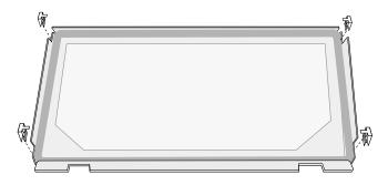
Figure 31. Use small pliers remove the four clips.
