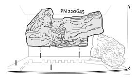
Figure 21. Engage the holes in the underside ot the Rear Log with the two pegs in the burner skirt.
