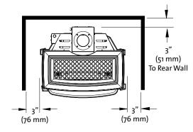
Figure 2. Parallel Installation Clearances.
