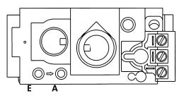
Figure 19. Pressure test points.
