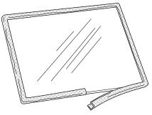
Figure 32. Wrap the gasket around the glass panel.
