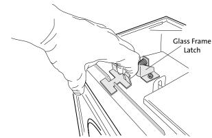
Figure 48. Release the glass frame latches.
