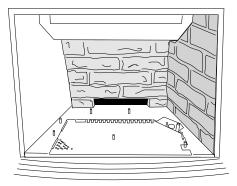
Figure 50. Install the Side Panels.
