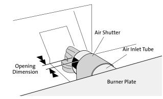
Figure 15. Air Shutter Setting
