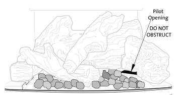
Figure 24a. Position embers loosely and maintain 1/4" clearance from the burner skirt edges.
