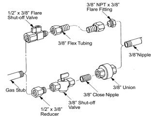
Figure 18. Supply valve connection fittings.
