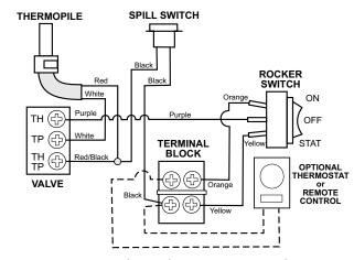
Figure 26. B-vent valve and accessory wiring diagram.
