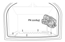
Figure 20. Engage the holes in the underside ot the Right Log with the peg in the burner skirt.
