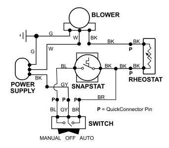
Figure 37. Blower Wiring Diagram
