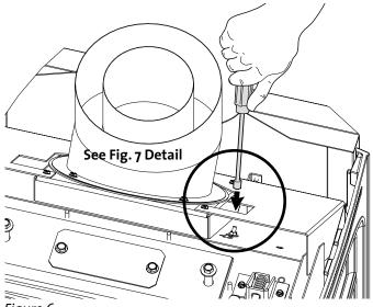
*Figure 6. Use a nut driver to change the Exhaust Restrictor setting.*
