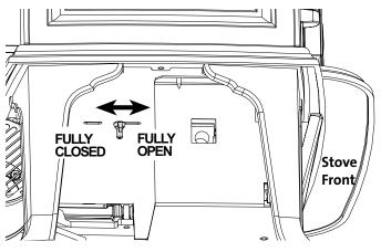
Figure 21. Locate and loosen the Air Shutter wingnut under the stove.
