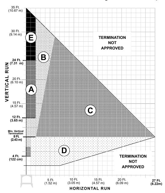
Figure 8. ZONE E: For terminations between 24-35 feet. Install Exhaust
