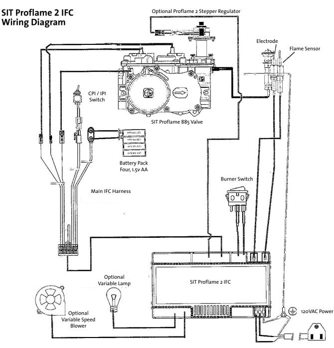
Figure 71. GF 300 DV IPI Allagash with Proflame 2 Premium Remote Control Accessories
