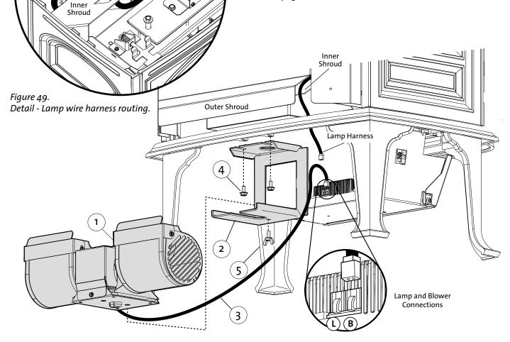
Figure 50. 157470 Blower Kit Components used for GF 300 DV IPI Allagash.
