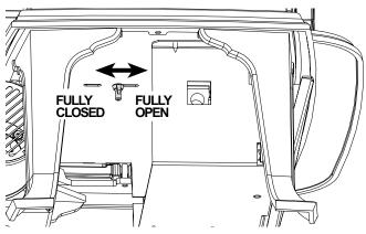
Figure 42. Loosen the wingnut to adjust the air shutter.
