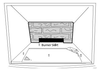
Figure 30. Install the Lower Rear Panel.
