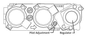
Figure 41. Manual flame regulation.
