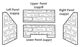
Figure 29. Panel kit components.
