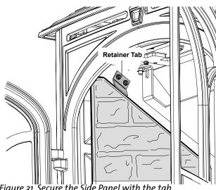
Figure 31. Secure the Side Panel with the tab.
