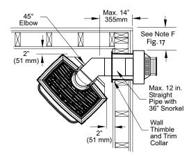
Figure 20. Corner Installation with 36" Snorkel Termination.
