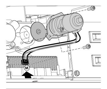
Figure 47. Flame Control Motor installation.
