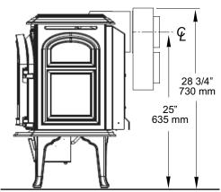
Figure 12. Simpson Dura-Vent #923GCL Co-linear Adaptor. Subtract 2 1/4" for Short Legs.
