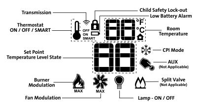
Figure 52. Remote transmitter display data.
