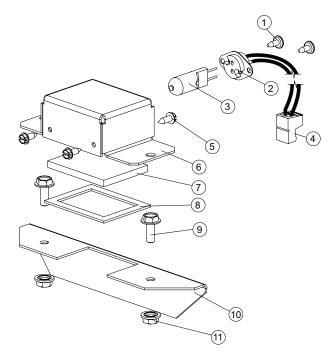
Figure 75. GF 300 DV IPI Accent Lamp Assembly
