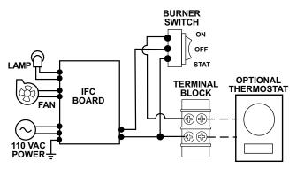
Figure 40. Accessory wiring diagram.
