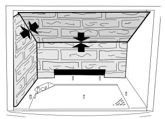
Figure 32. Install the Upper and Side Panel.
