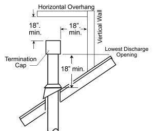
Figure 10. Vertical vent termination height above roof.
