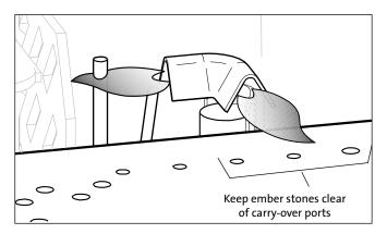
*Figure 39. Proper pilot flame appearance relative to burner carry-over porting.*
