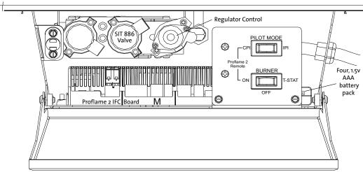
*Figure 44. Control Compartment.*
