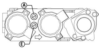
Figure 27. Pressure test points.
