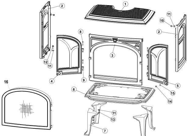
Figure 72. GF 300 DV IPI Cast iron parts and associated hardware, Version 2.
