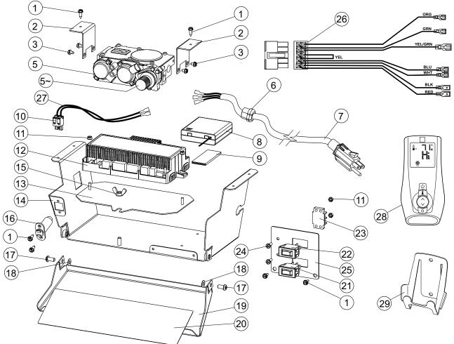
Figure 73. GF 300 DV IPI Valve Assembly and IFC Components.
