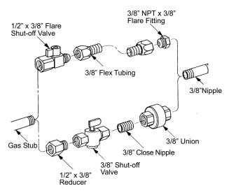
Figure 26. Supply valve connection fittings.
