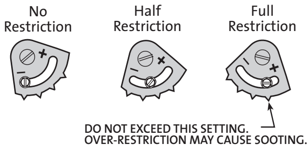
Figure 15. Exhaust Restrictor settings
