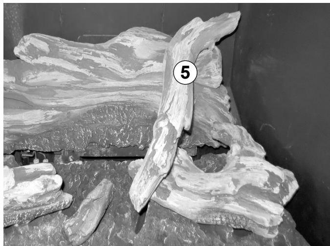
Figure 7.31. Engage indents in the underside of the Upper Right Log #5 with the matching marks on logs #1 and 4.
