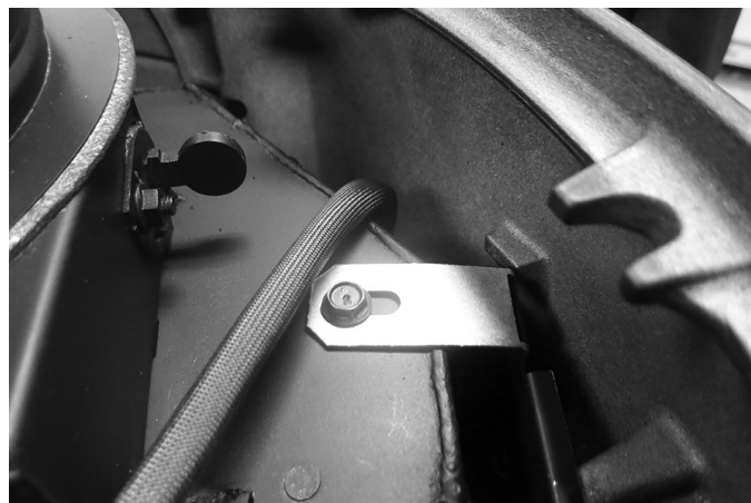
Figure 16.2. Remove the firebox-to-side plate bolt.
