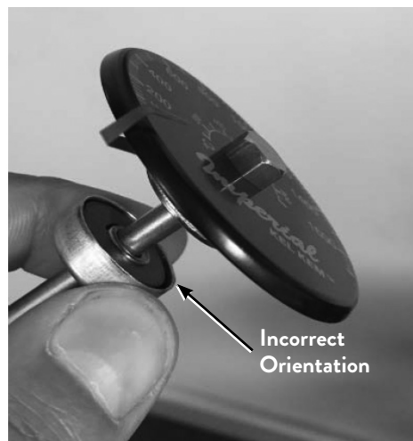
Fig. 13c. Remove magnet from current orientation
