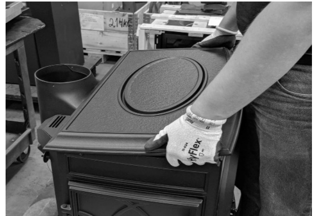
Fig. 21. Remove the top plate from stove.
