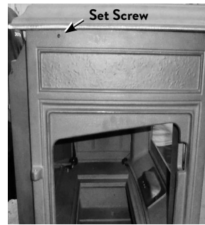
Fig. 20. Remove M6x40 set screws from left and right sides.
