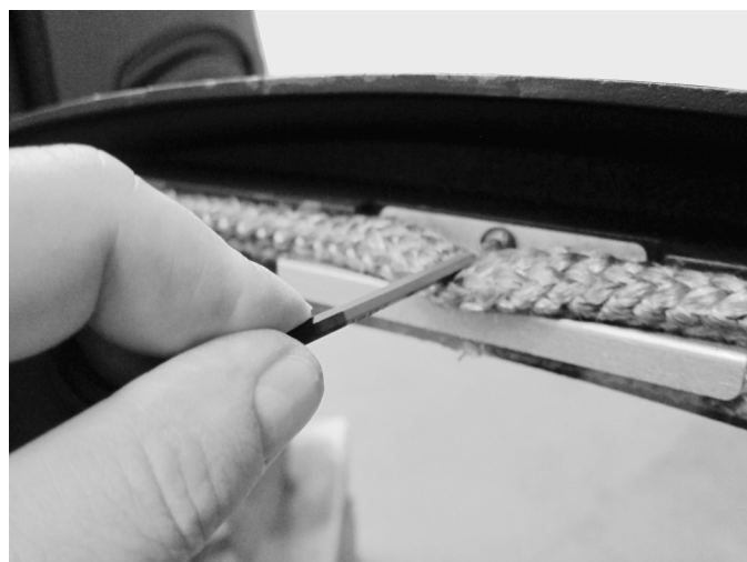
Figure 20. Loosen the glass clips.
