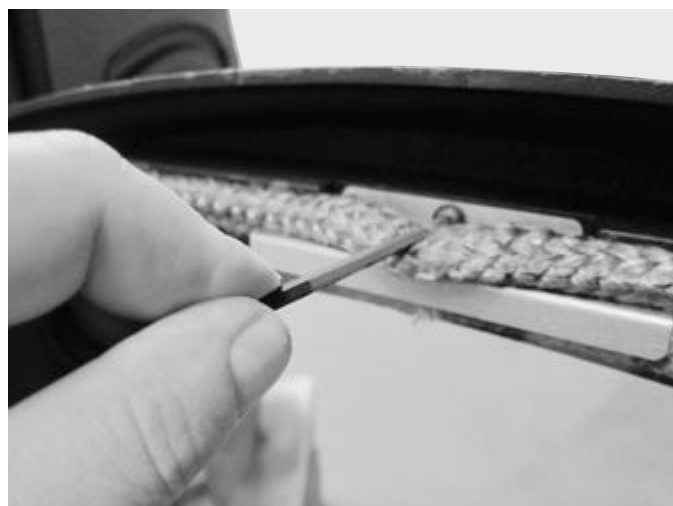
Figure 20. Loosen the glass clips.
