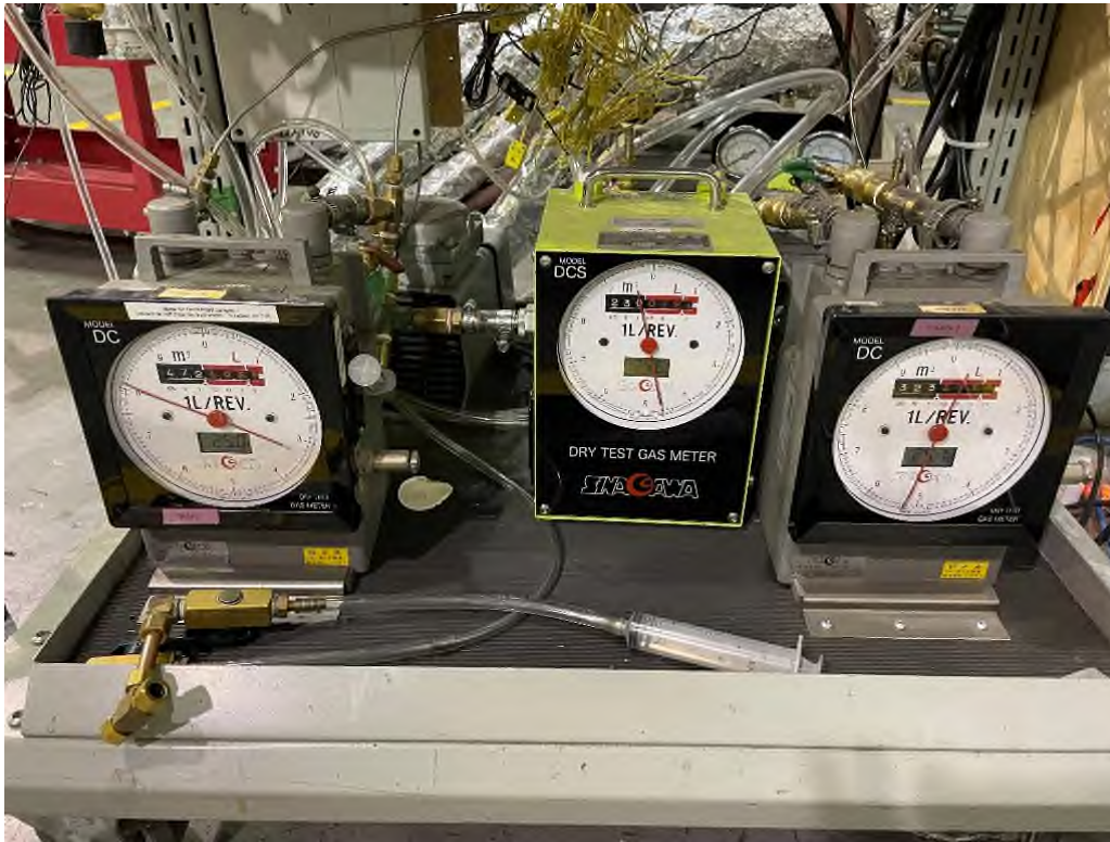
Picture 11: Dry gas meter
