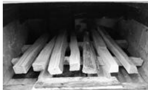
Figure 25. Arrange smaller fuel start-up pieces on top of grid
