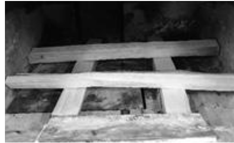
Figure 24. Arrange larger fuel start-up pieces on bottom
