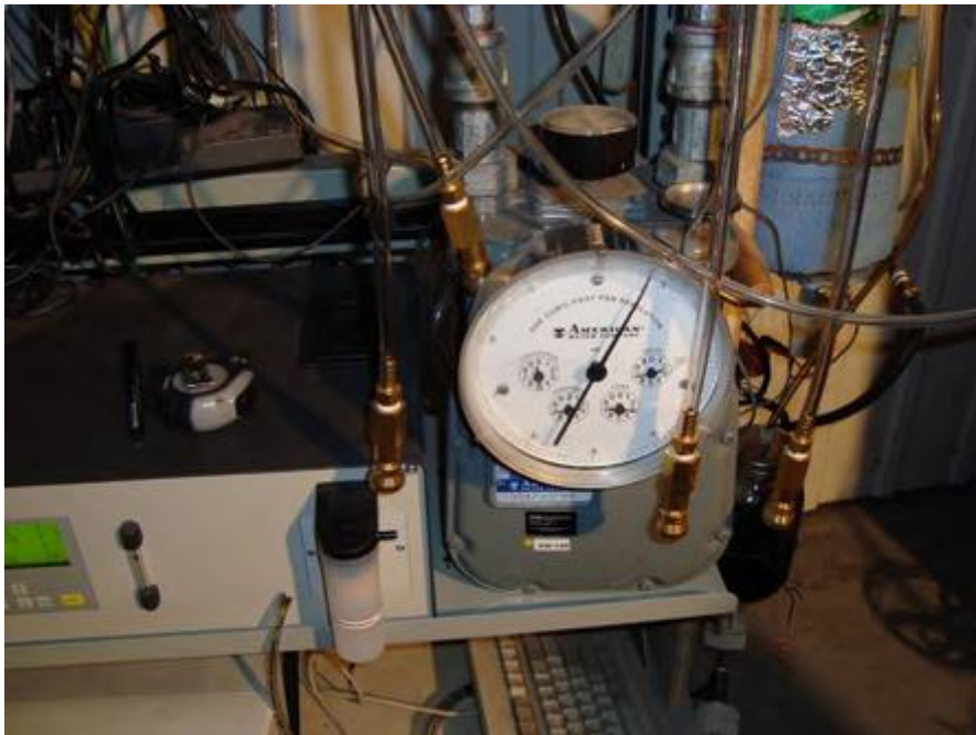
Picture 8: Reference dry gas meter
