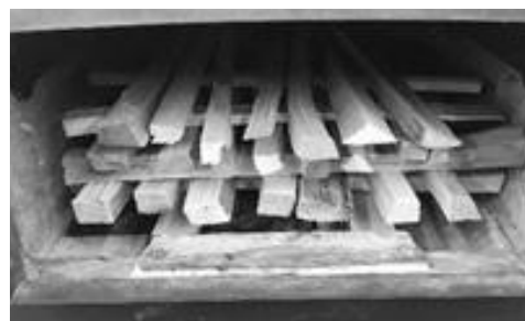
Figure 27. Arrange kindling in grid pattern on top
