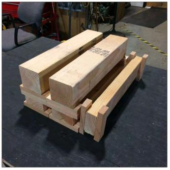
Typical Test Fuel Load Configuration
