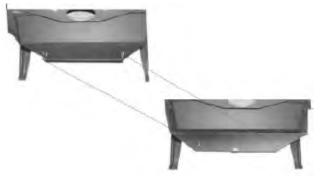
3) Oriented as shown, use the two bolts to attach the heat shield to the stove bottom.
