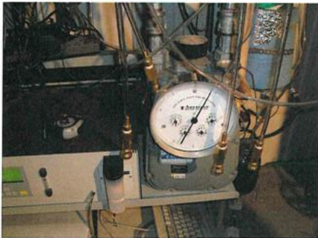
Picture 8: Reference dry gas meter
