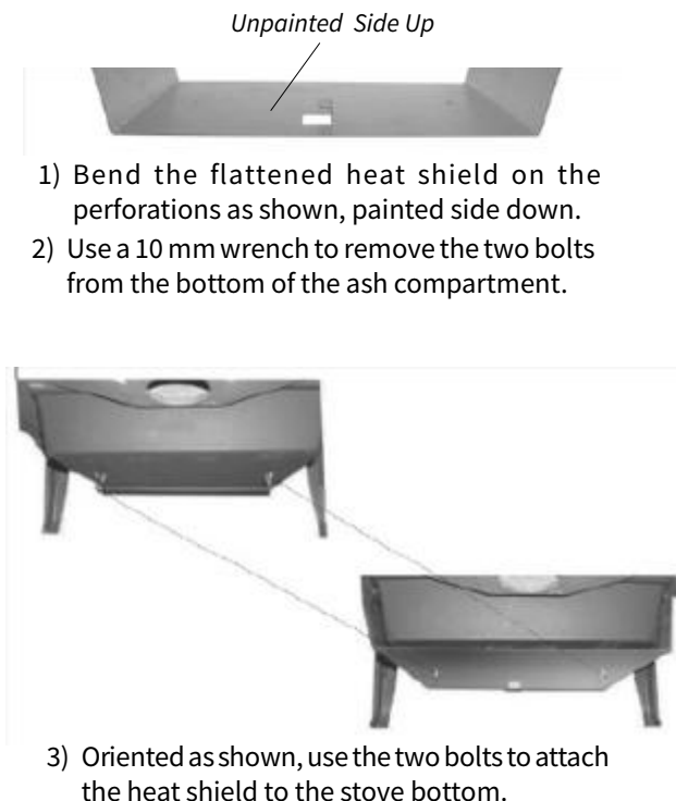
Fig. 4.3. Bottom heat shield installation.
