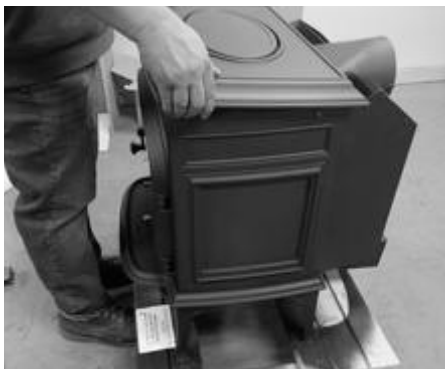
Fig.6.5. Remove the top plate from stove.
