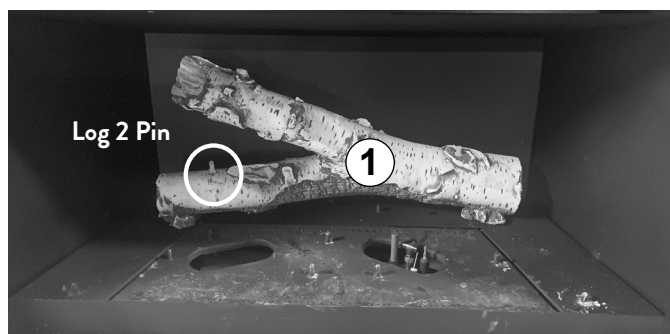
Figure 7.35. Engage the Rear Log #1 with the two steel pins located on rear burner skirt.
