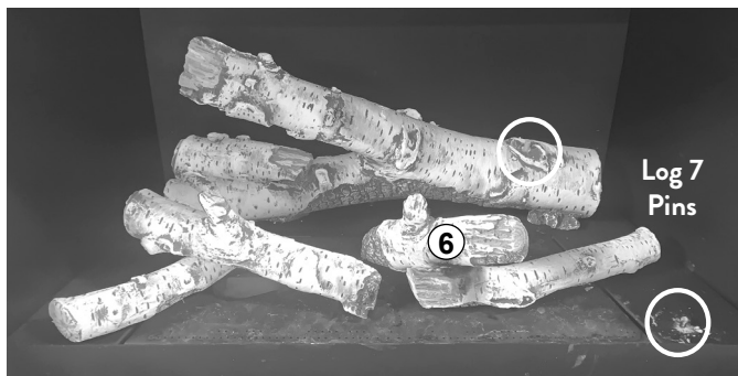
Figure 7.40. Engage matching notches in the underside of the Middle Cross Log #6 with the corresponding pins on Log #4 and the burner indicated in fig. 7.39.
