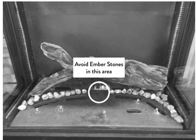
Figure 11.2. Place 12-15 Ember Stones on each side of the Burner. Avoid the Pilot carry-over area.
