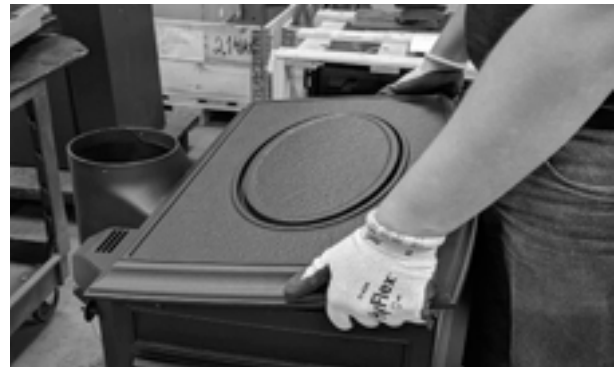
Fig. 21. Remove the top plate from stove.
